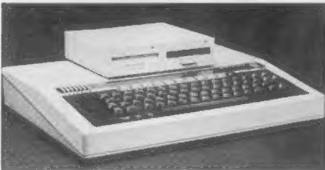
Hitachi's dual 3in disc drive perched on top of a BBC micro
